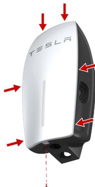
3. Use a T10 Torx driver to install the screw that secures the bottom of the outer cover to the housing. Tighten the screw to 4.4 in-lb (0.5 N-m).
